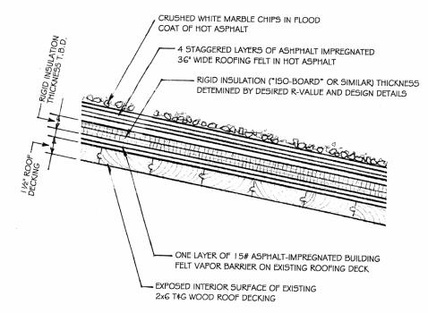
C. 4-PLY BUILT-UP ROOFING SYSTEM
