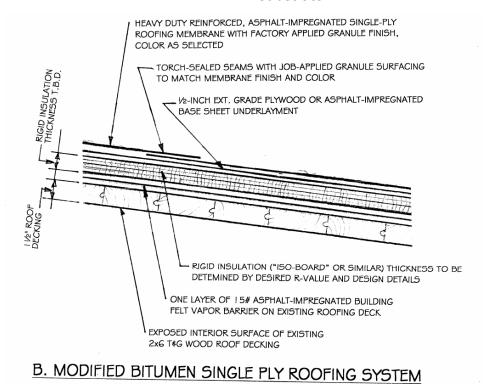
SBS membranes can be hot asphalt applied, torch applied, or cold process applied. The black ooze that emanates from heat-sealing the seams can be minimized and covered with powdered surfacing matching roofina the eliminate any unsightly detraction from an otherwise viable roofing system.
